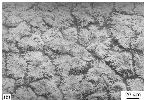
Figure 7 SEM micrographs showing the effect of LPE content on the morphology of blends crystallized at 124°C: (a) 3% LPE; (b) 15% LPE.
